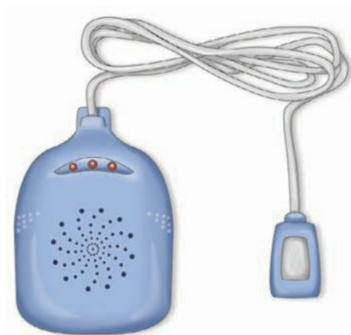
FIGURE 21.6 Some children and families find great success with the use of an enuresis alarm. The alarm wakes the child at the first sign of wetness. Over time, the child learns to awaken at night in response to the sensation of a full bladder.
