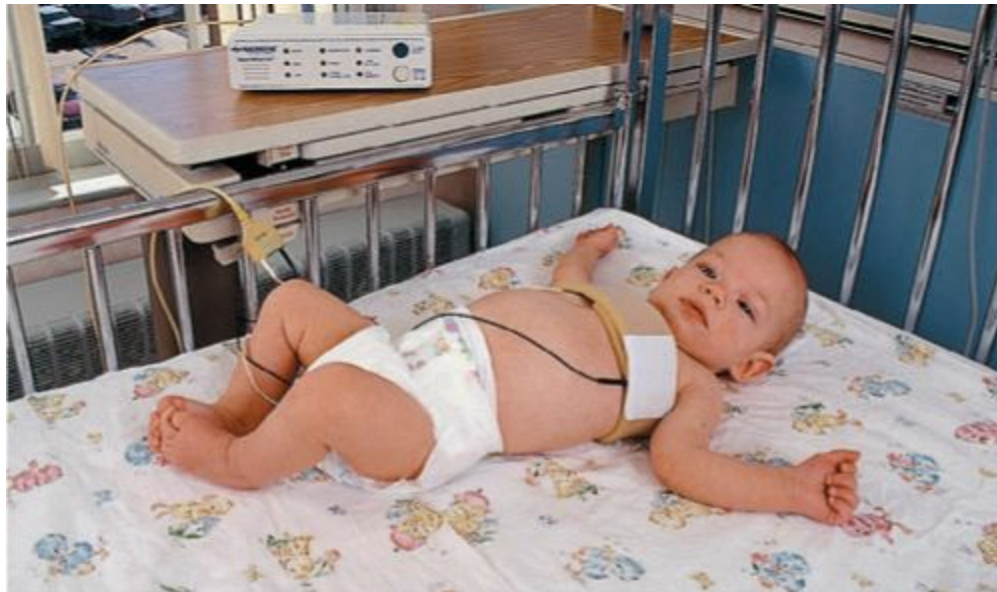
FIGURE 18.15 The home apnea monitor uses a soft belt with a Velcro attachment to hold two leads in the appropriate position on the chest.
